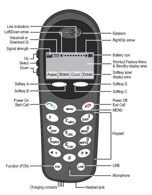
SpectraLink 8002 Wireless Telephone
